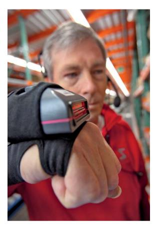
The 'Pick Execution<sup>™</sup> System' from Numina uses wireless barcode scanners, which are worn on the wrist and are characterized by the greatest possible flexibility and ease of use.
