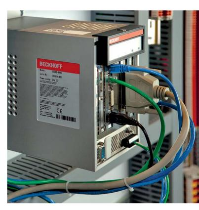
The backbone of the control system is a Beckhoff C6340 Industrial PC, equipped with an Intel<sup>®</sup> Pentium<sup>®</sup> M 1.8 GHz processor.
