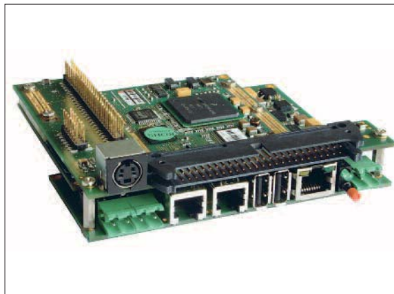
Figure 1: Power architecture MPC5200 CPU module with carrier board and typical physical connections
