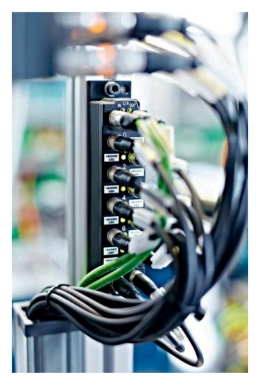
In the process, decentralized collection of I/O data via the EtherCAT Box modules, EP1008 and EP2028, directly on-site reduces the required control cabinet space to a minimum.
