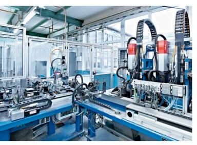
The interlinked key production line designed by Aumat and AST, consisting of a key cutting machine and a profile milling machine, machines key blanks with high precision down to lot size 1.
