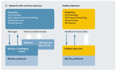
Figure 3. IT and fieldbus networks have quite a few different properties
