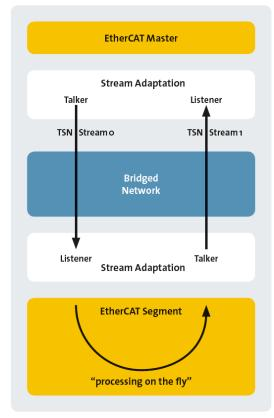
Figure 5. Stream adaptation and TSN provides a virtual Ethernet channel
