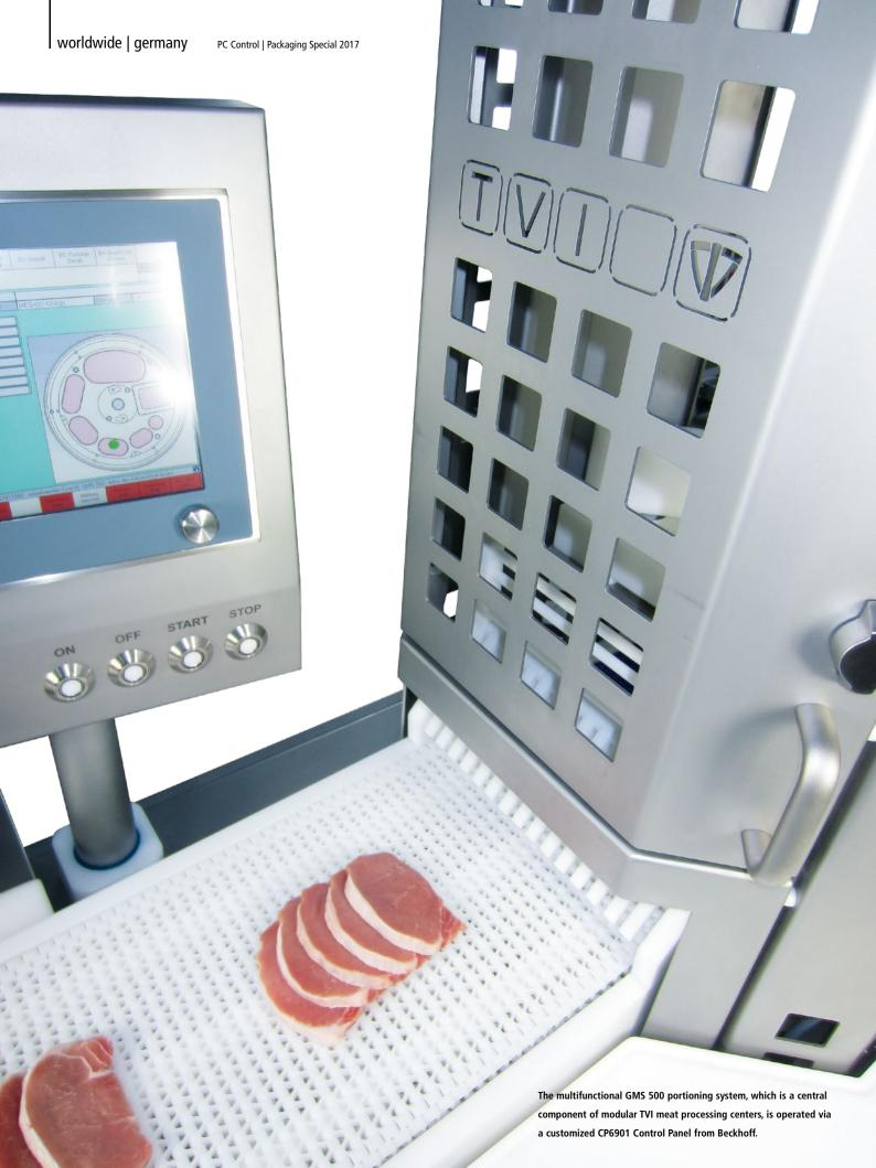
PC-based control and servo drives form the basis for highly accurate weight-based meat portioning
