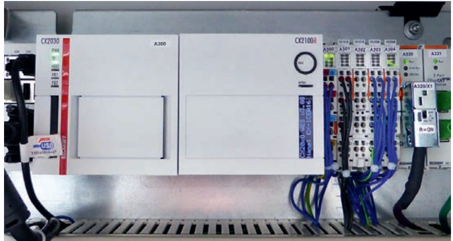
The CX2030 Embedded PC and TwinCAT 3 software form the core of A10 stacker's automation solution.
