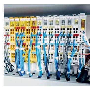
With the TwinSAFE terminals (left) and the EL7201 servomotor EtherCAT Terminal (right), extremely compact safety and drive technology can be integrated seamlessly into the control system.
