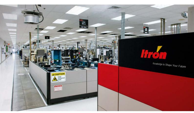
To meet the rising demand for gas and water metering devices, Itron has upgraded the assembly cells in its Waseca, Minnesota plant to PC- and EtherCAT-based control systems.
