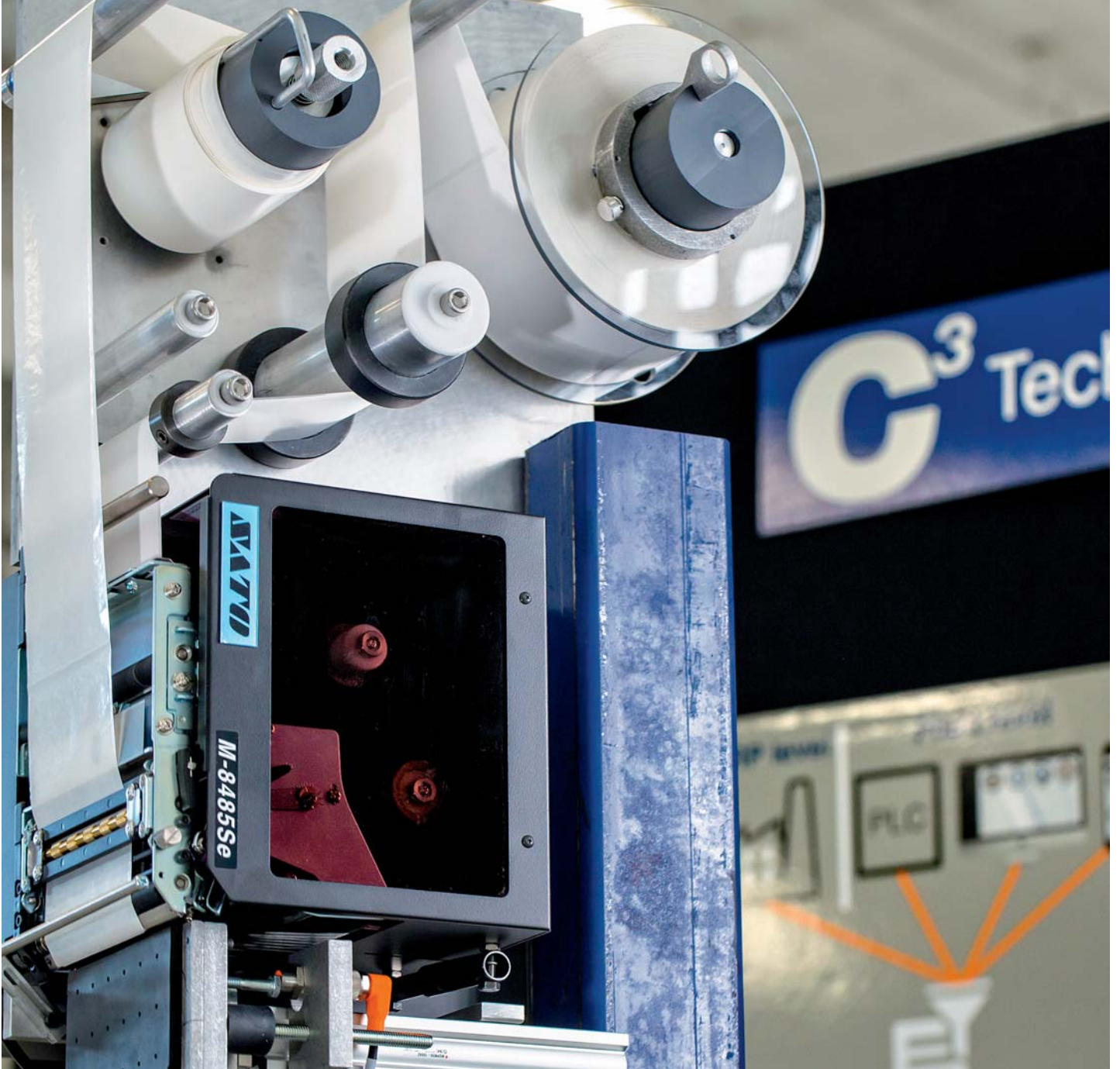
The Smart Identity System from C 3 features extensive connectivity. Users can issue commands, run diagnostics, change templates and labels, and access data from any web-capable device.
